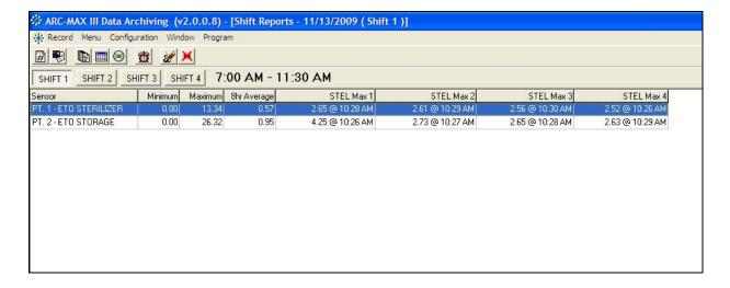
The shift report shows the minimum, maxium and average gas concentration values for the duration of the shift as well as the four highest STEL values logged during the shift and the times each STEL ended. NOTE: Should the data regions not appear in the report as they do in the example above and data appears missing, simply drag the region boundary to the right to expand the data column.
