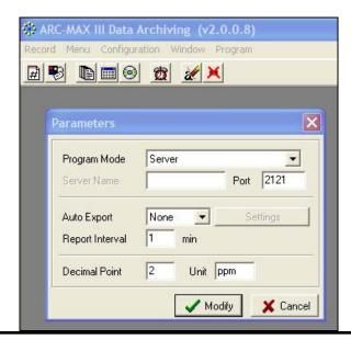
**Program Mode:** This parameter sets how the program operates in relation to the PC it is running on. If you chose "Server" in this field, the program will run in server mode as the primary "host" to all other instances of the program, if any. All system settings, configuration and data log manipulation will be accessible to the user.
