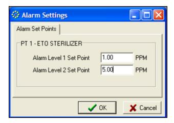
To change an alarm set point value, click in the desired field and change the value by backspacing to erase the previous value and typing in the new value. Click "OK" when finished to save the new value. Repeat as needed for additional channels.
