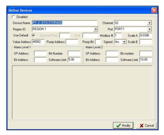
ONLY THE "DEVICE NAME" PARAMETER SHOULD BE CHANGED BY THE USER UNLESS DIRECTED TO DO SO BY **INTERSCAN**. To change the DEVICE NAME, click in the DEVICE NAME field, backspace over the old name and type in the desired name then click **Modify** to save the changes.
