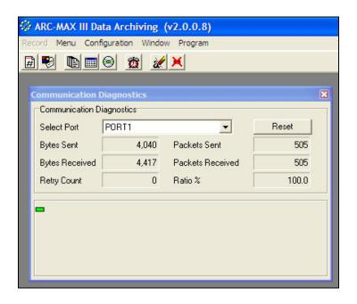
The status of each Port is displayed graphically in the lower half of the Communications Diagnostics window – to give the user a quick overview of attached devices. A colored rectangle represents each port accessed. A white rectangle indicates that device status is not yet determined. A green rectangle indicates device communications are good. A red rectangle indicates a device communications error. A yellow rectangle indicates that the device communication status is currently being updated.
