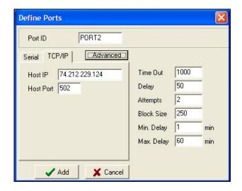
To create a new Port ID, right click anywhere in the Define Ports window and select New. A Port ID must be input in order to create a new record. Select the serial Tab to set the Com Port and Baud Rate settings for serial connections or select the TCP/IP tab to enter Ethernet settings for Ethernet connections. The Advanced option allows user to edit Time Out, Delay, Attempts, Block Size, Min Delay and Max Delay values.
