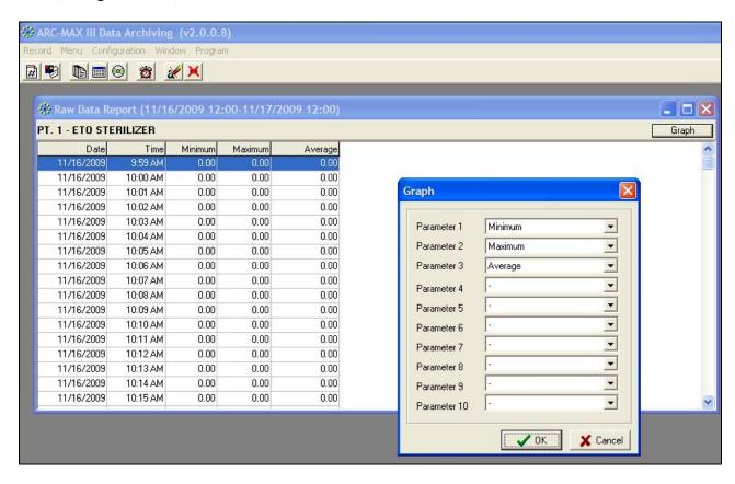
Here you can select any or all of the three data values shown in the Raw Device Report to be displayed in graphical form. Click on any parameter window to select the desired data value for that parameter. The default settings are Parameter 1=Minimum, Parameter 2=Maximum, Parameter 3=Average. If you only wish to view one of the three values (for example, Maximum), you must set that value in the first parameter window and select a blank setting for the other two parameters. (see below).
