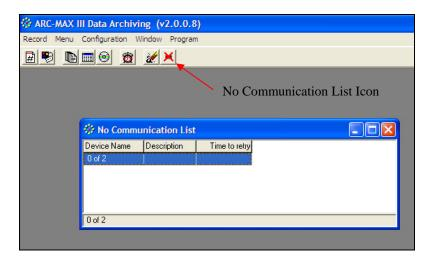
To troubleshoot channels that may not be communicating with the software, click on the "No Communication List" icon or select **No Communications List** from the drop down MENU list. This will open a window that displays the Device Name, Description and Time to retry connection of each device not communicating. Right clicking a device on the list allows the user to restart communications via "Retry Now", or view devices by region via "Show Regions".
