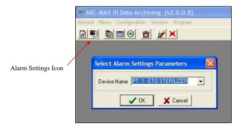
To open the Alarm Settings page from the tool bar click on the "Alarm Settings" icon shown above or select **Alarm Settings** from the drop down MENU list.
