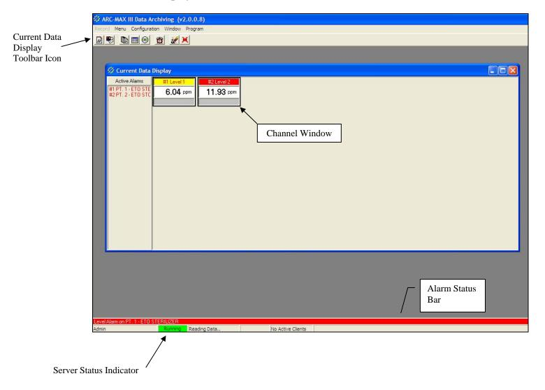
To open the Current Data Display from the tool bar, click on the Current Data Display icon as shown above or select **Current Data Display** from the drop down MENU list.
