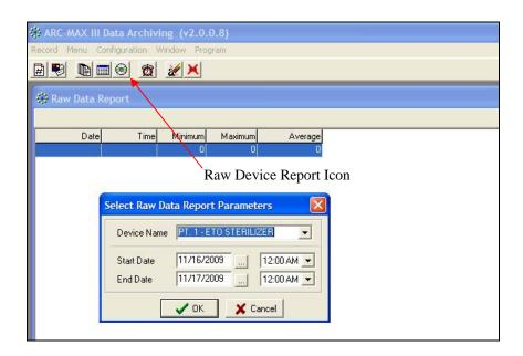
The report generated will show Min, Max, and Avg data values for each minute of the time period selected. (see figure below). Depending on the size of the time period selected, the data may be displayed in a full screen window that will require scrolling.
