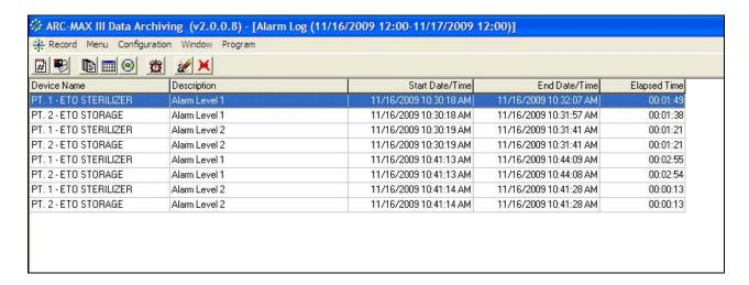
The alarm log records device name, alarm description (level), date/time of start of alarm event, date/time of end of alarm event and duration of alarm event as shown in the figure above.
