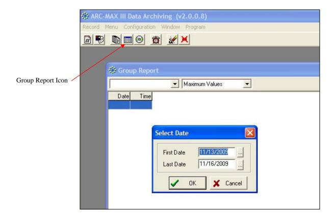
The report will display data for the channels selected when the last group report was generated. (See section 2.4.1, pg 10 for new channel selection instructions). Select the period between each displayed data set via the left side drop down box (minutes/hours/days – "minutes" shows as a blank selection). Select the data content to be displayed from the right side drop down box (Minimum/maximum/average value).
