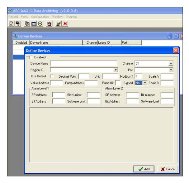
The Device Name, Region ID, Channel, Port, Value Address, Scale A, Decimal Point and Unit values must be input in the associated fields in this window. Contact the Interscan Systems dept for the correct values to enter in these fields for your application. Once these values are entered, click **Add** to save the values and create the new channel device.
