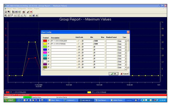
NOTE: It's a good idea to check the configuration with each graph viewing to ensure the labels and scaling setup match each parameter selected when the graph was opened. This is particularly important when viewing GROUP report graphs when the channels displayed are changed from previous graphs or after altering the channels populating the group.
