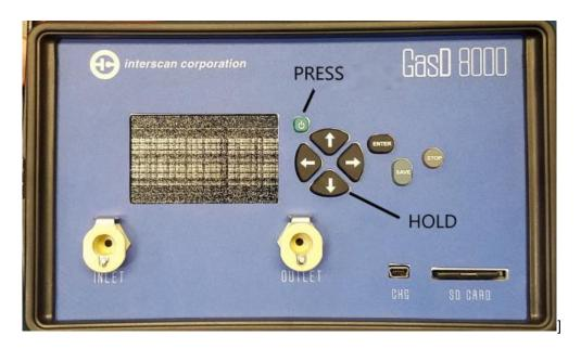
NOTE: Sometimes when manipulating multiple buttons on the keypad with one hand, an edge of a button may become stuck under the panel overlay. Should you notice this has happened, simply lift the stuck edge gently away from the panel to free it. Do this before proceeding.
