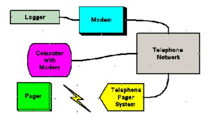
The logger is connected to a modem with a "logger to modem" cable (this is a different cable to the <u>Download</u> <u>Cable</u>). The modem is connect to the telephone network. The logger can now be controlled by any computer with a modem that is connected to the telephone network. The logger can also be configured to send a message to a pocket pager on the telephone network if user specified alarm conditions occur.
