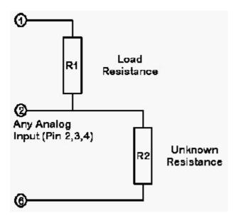
The Omnilog software needs to know the exact value of R1, the load resistor.
