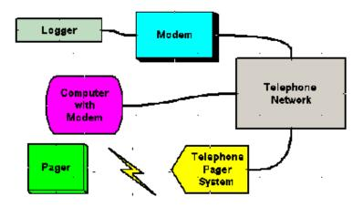
The logger is connected to a modem with a "logger to modem" cable (this is a different cable to the Download Cable). The modem is connect to the telephone network. The logger can now be controlled by any computer with a modem that is connected to the telephone network. The logger can also be configured to send a message to a pocket pager on the telephone network if user specified alarm conditions occur.
