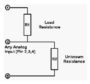
The Omnilog software needs to know the exact value of R1, the load resistor.
