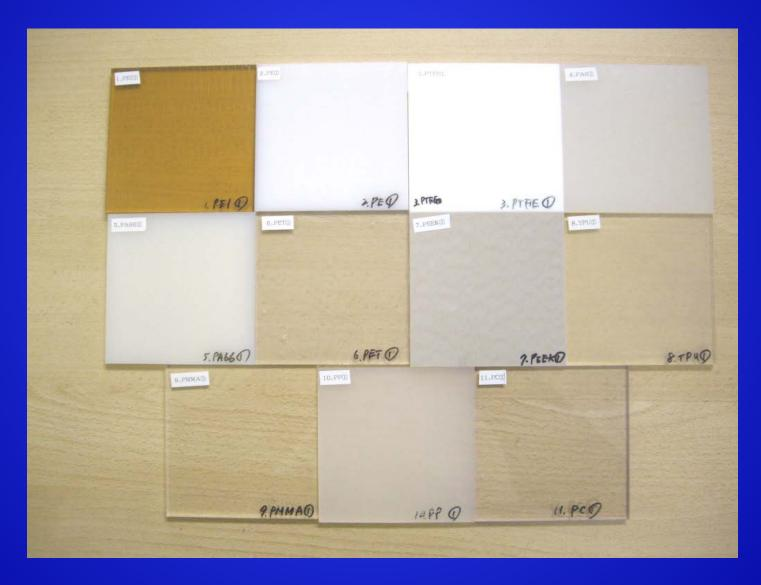
Eleven Kinds of Plastic Test Panels100mm × 100mm × 6mm Detection 1 × /10sec. for 25min.
